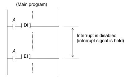
El and DI instructions should not be used in interrupt program. Also, these instructions should not be executed in the first scan.
